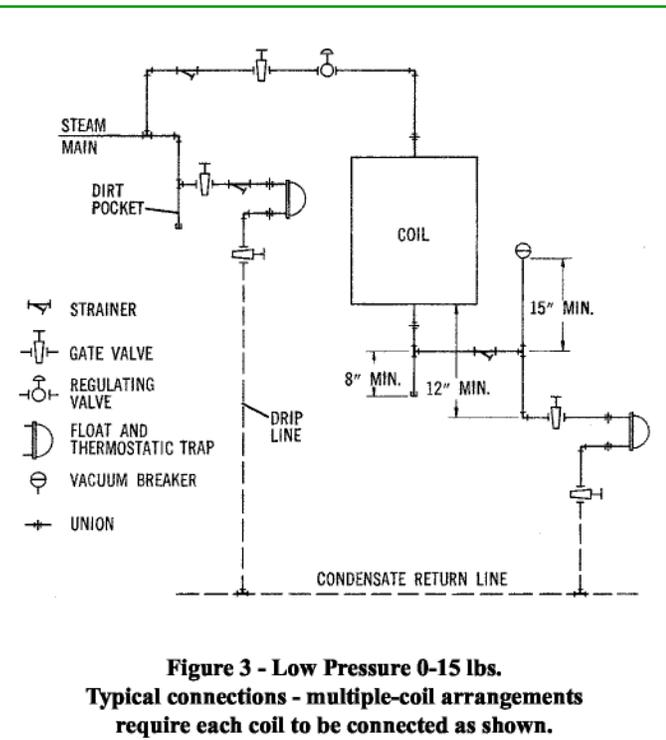
**Figure 3 - Low Pressure 0-15 lbs. Typical connections - multiple-coil arrangements require each coil to be connected as shown.**
