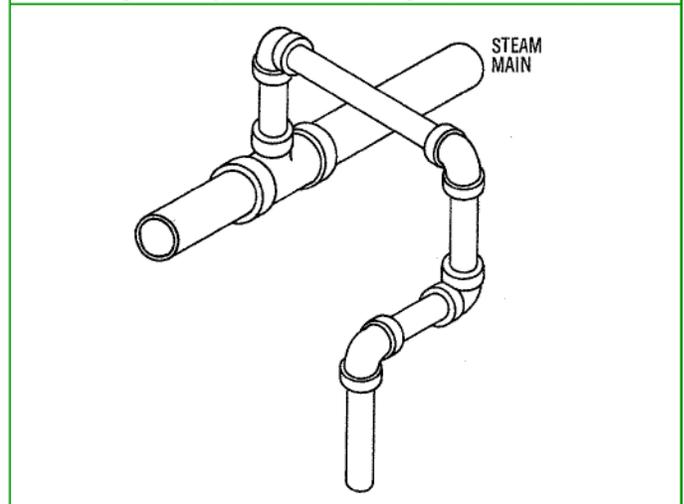
**Figure 6 - Typical Swing Connection**
