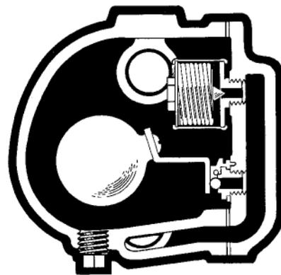
Float and Thermostatic Trap (Courtesy of Sarco Co.)
