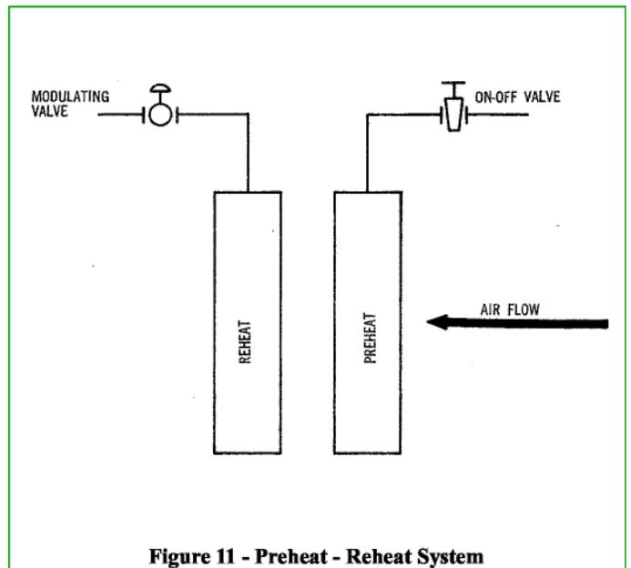
E. **Combinations** can be made of preheat-reheat with face and bypass. Fresh air and recirculating dampers may be used to exercise some control by closing down on fresh air in cold weather. Caution should be used in designing combination systems. Complex control systems are often maintenance headaches. Keep it simple.
