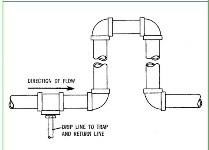
**Figure 5 - Typical Steam Piping Expansion Loop**
