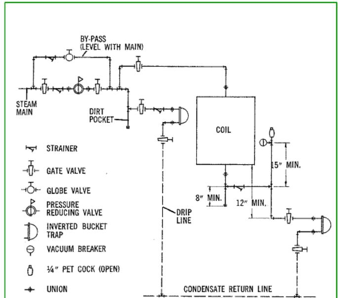
**Figure 4 - High Pressure 15 or more lbs. Typical connections - multiple coil arrangements require each coil to be connected as shown, except for the pressure reducing valve and by-pass line which is used only once ahead of a system.**
