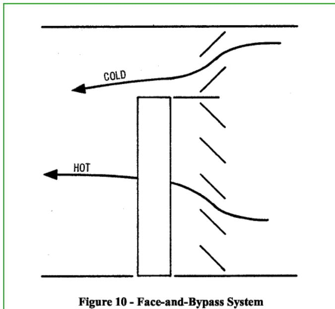
assume that summer operation will be with the steam off and air flowing through the face. Most customers seem to prefer low unit height to full bypass capability.
