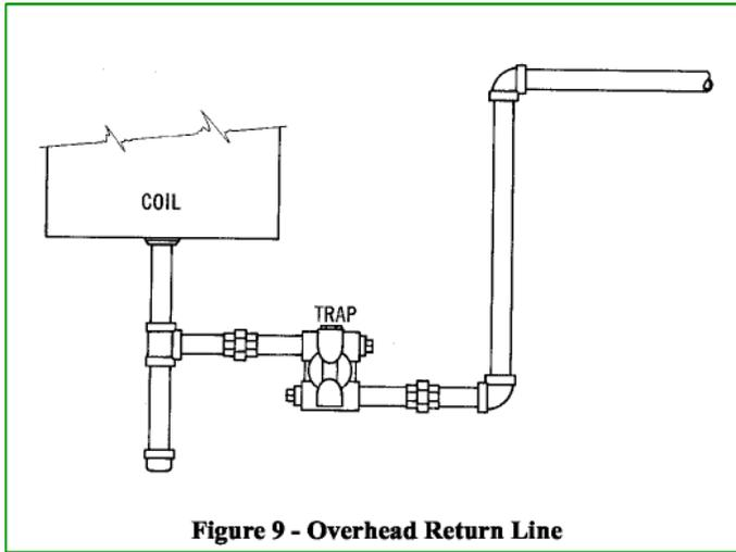
4. The traps, described in a previous section, must be installed below the coils. Water flows downhill. Overhead return lines (Figure 9) are perhaps the biggest single cause of freezing, water hammer, coil corrosion, and trap failure.
