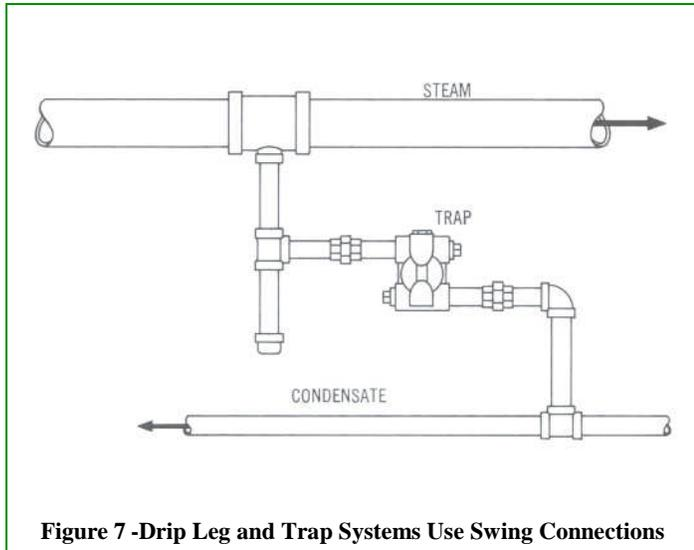
**Figure 7 -Drip Leg and Trap Systems Use Swing Connections**
