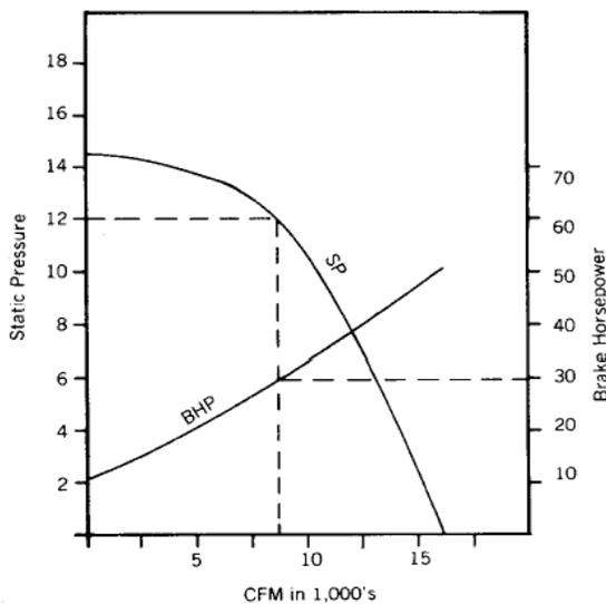
**Figure 1 - At 12" WG, the fan delivers 8750 CFM with 30 BHP. At 6" WG, the fan handles 13,000 CFM at approximately 44 BHP.**
