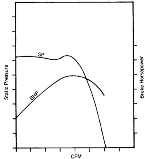
**Figure 2 - "Non-overloading" BHP characteristic inherent in backwardly-inclined wheel designs.**
