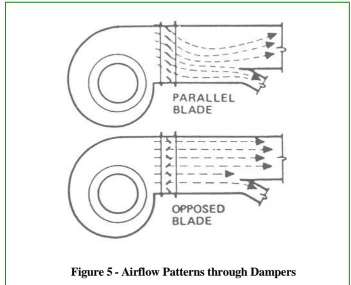
Figure 5 - Airflow Patterns through Dampers
