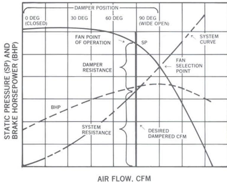
**Figure 1** - Static pressure and brake horsepower curves for backwardly-inclined fan with outlet damper. As the damper closes, the point of operation - brake horsepower and static pressure - moves to the left of the original fan selection point to the 90-degrees (wide open) damper setting.
