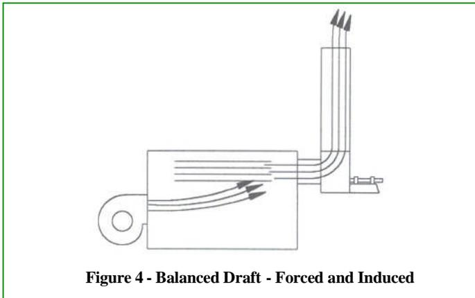
**Figure 4 - Balanced Draft - Forced and Induced**
