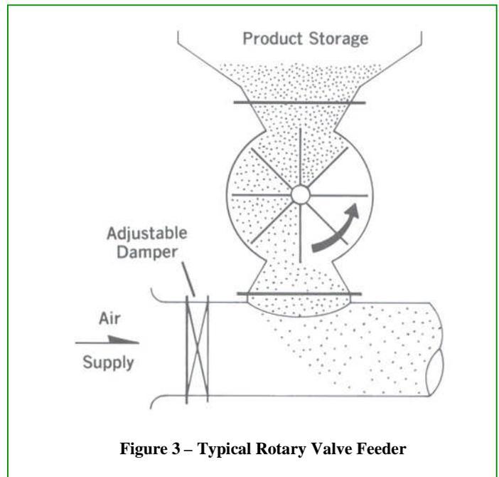
**Figure 3 – Typical Rotary Valve Feeder**
