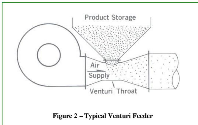
**Figure 2 – Typical Venturi Feeder**
