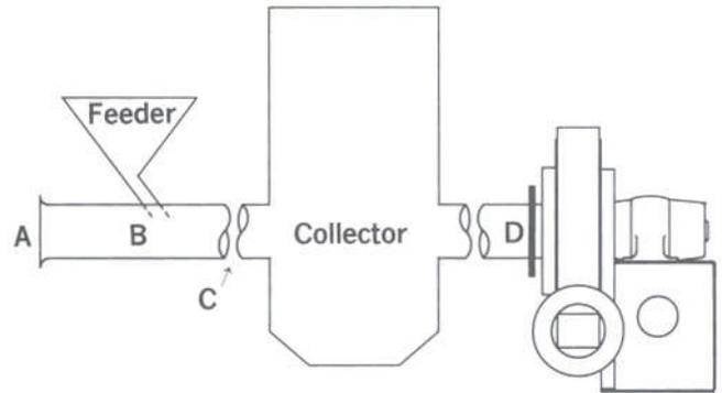
Given: draw-thru pneumatic conveying, as illustrated.
