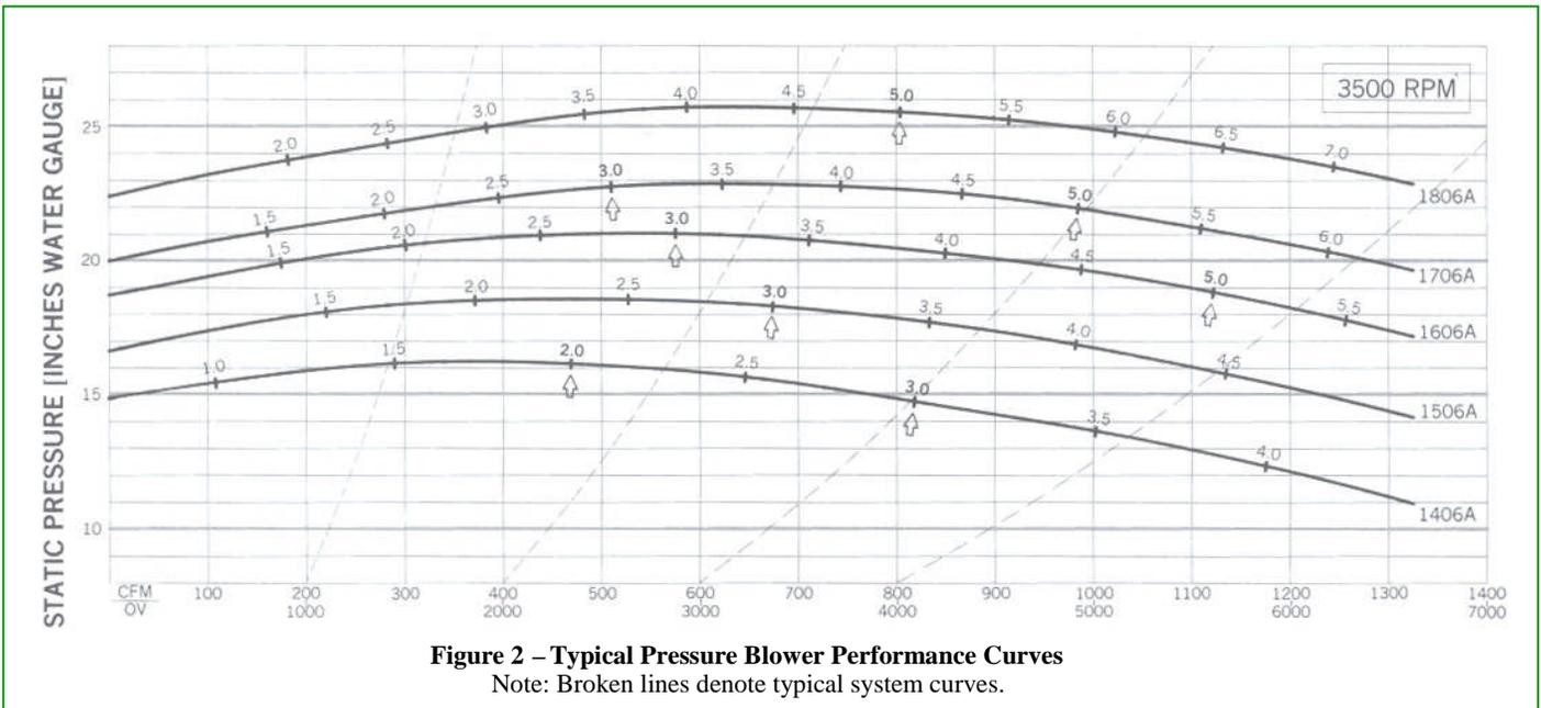
**Figure 2 – Typical Pressure Blower Performance Curves**
