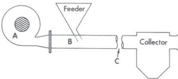
Given: injector conveying system, as illustrated.
