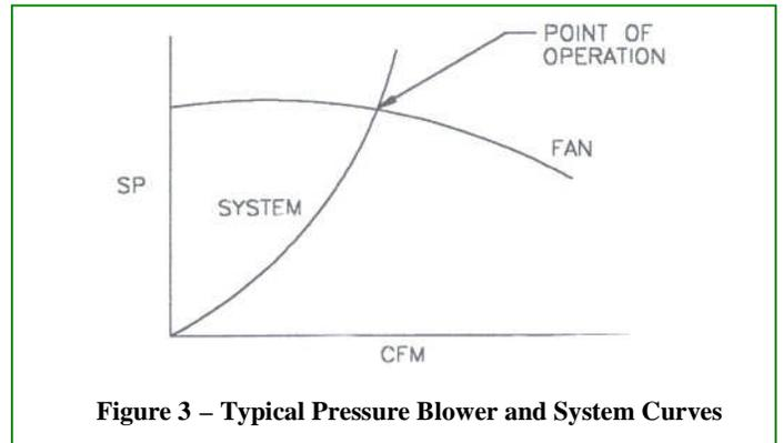
**Figure 3 – Typical Pressure Blower and System Curves**
