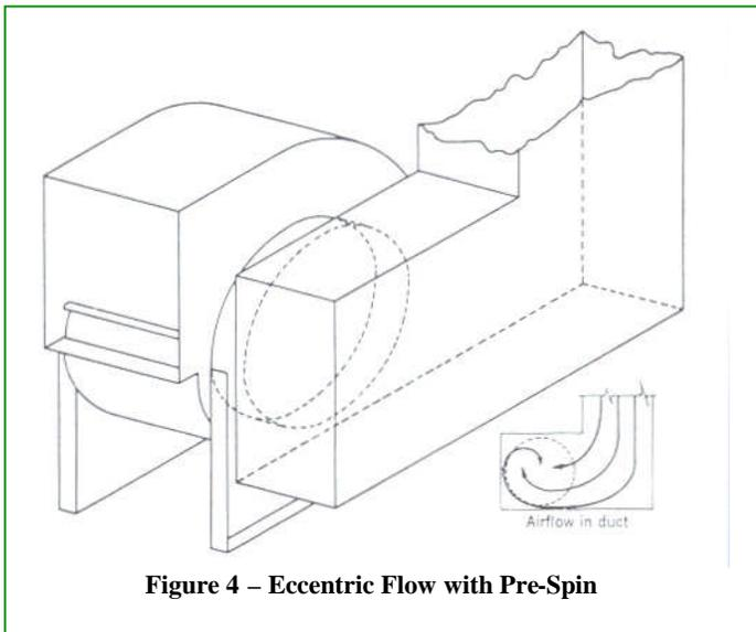
Figure 4 – Eccentric Flow with Pre-Spin
