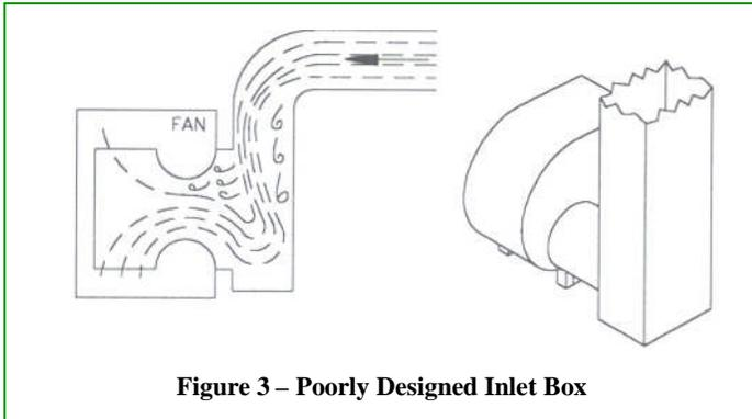
Figure 3 – Poorly Designed Inlet Box
