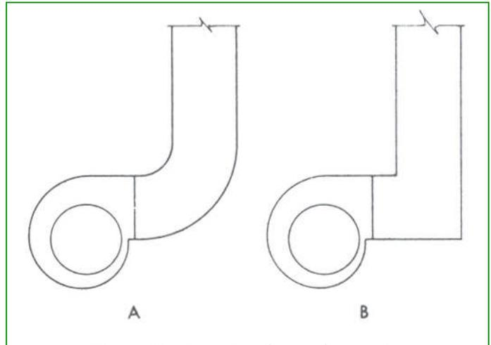
**Figure 10 - Poor Fan Outlet Connections**
