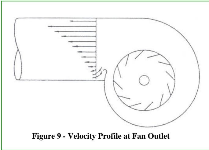
**Figure 9 - Velocity Profile at Fan Outlet**
