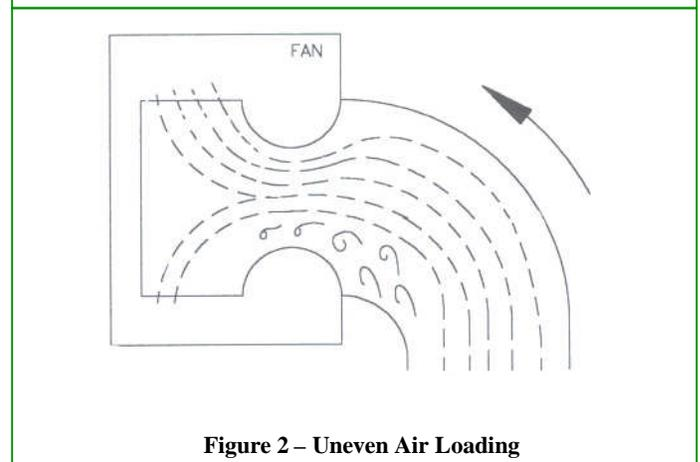
Figure 2 – Uneven Air Loading
