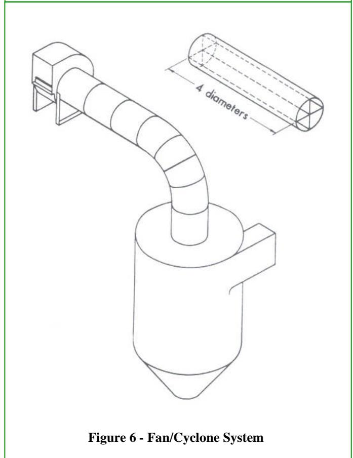
Figure 6 - Fan/Cyclone System
