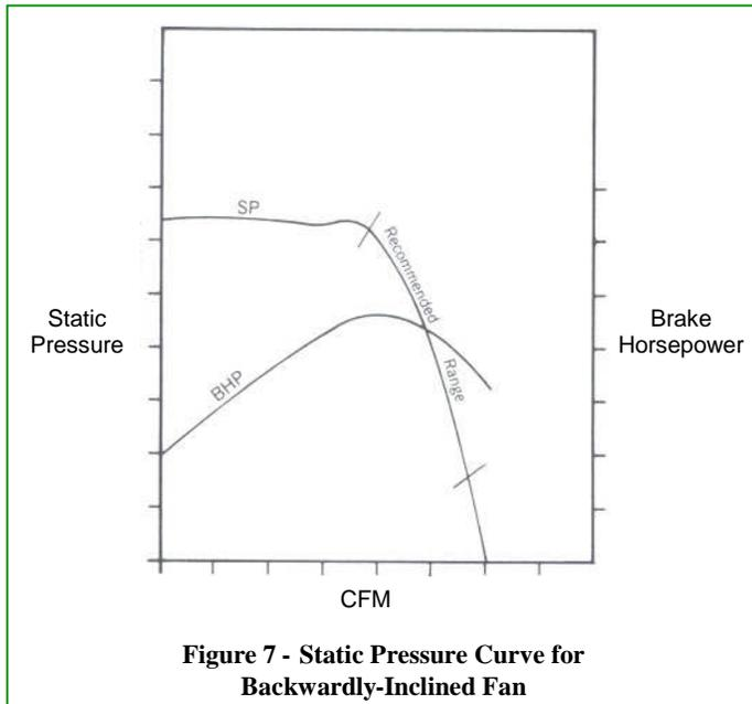
Figure 7 - Static Pressure Curve for Backwardly-Inclined Fan
