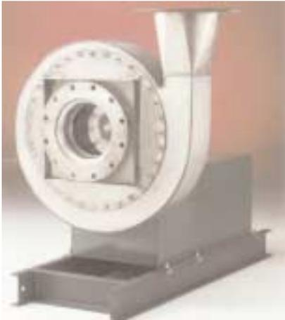
Pressure Blower with stainless-steel airstream and high-build epoxy-coated structure for landfill-methane evacuation.
