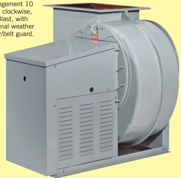
Arrangement 1 GFE, clockwise, Bottom Angular Up, with optional inspection port, unitary base, discharge damper, outlet flange drilling, motor, and guards.
