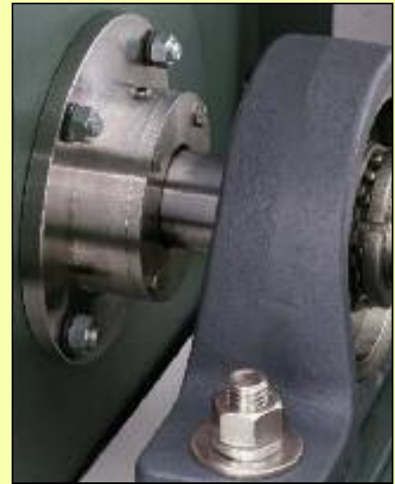
Gas-purgeable double carbon ring shaft seal.
