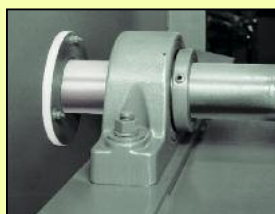
450°F. design ceramic felt shaft seal.
